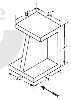
The figure represents a symmetrical metal casting with horizontal rectangular base and top. All parts are  $\frac{3}{8}$  in. thick. Draw, full size, the plan and an elevation in the direction shown.
